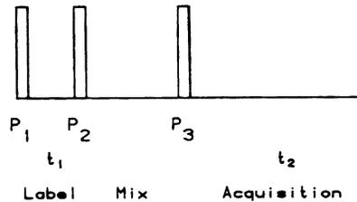
FIG. 1, The pulse sequence used in two-dimensional spin exchange spectroscopy.  $P_1$  and  $P_2$  are two  $\Pi/2$  pulses used to label spins in the  $t_1$  dimension. The spins are allowed to mix and a final detection pulse  $P_3$ , is applied to excite a free-induction decay during  $t_2$ .
